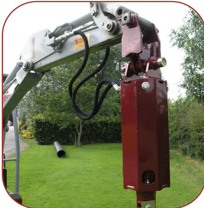
4. De-pressurise hydraulic systems using the manufacturers approved techniques before connecting the Powerhead.
