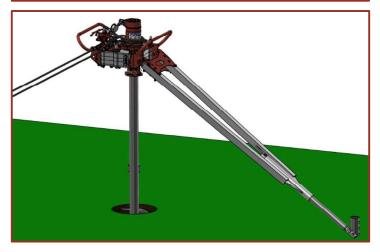
11. Continue to install the screwpile until the desired height is reach or the 700H reaches ground level.
