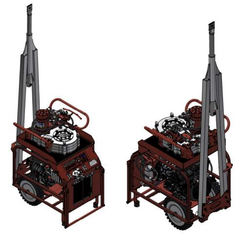
If being transported separately from an Autoguide Equipment powerpack, it is recommended to remove the driver to ensure the machine sits flat and is stable.
