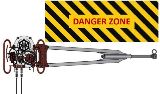
6. Ensuring that the immediate vicinity is clear of bystanders, and that there is nobody in the 'Danger Zone' highlighted above the screwpile can be installed. Using the handle to operate the 700H, install the screw pile until torque head reaches ground level.
