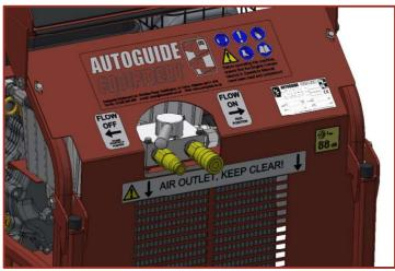
5. First connect the return line to the powerpack, followed by the pressure line. Ensure the quick couplers seal and twist to secure.
